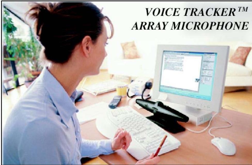
Unlike 1st generation array microphones which have a fixed "listen" direction, the Voice Tracker™ Array Microphone automatically locates and electronically steers toward the talker.
